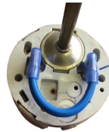
Figure 4.4 Bridging wire fitted to TSE Thermostat
