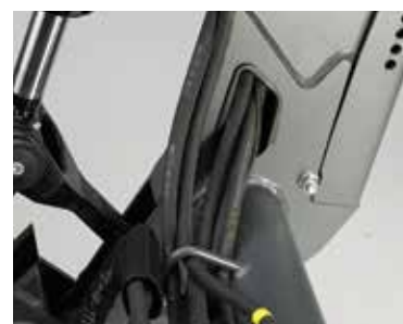
3 | NEW! PROTECTION OF THE HOSES IN THE LOADER BEAM ACCESS.
