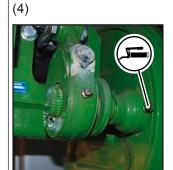
Use a different lubricating grease for this lubrication point, see Page 53.
