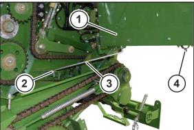
To secure the twine box (1) in the unfolded position, insert the wire bracket (3) from the mounting bracket (4) into the borehole (2).
