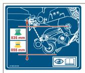
The height of the drawbar has been optimally set when the distance between the centre of the cutting rotor or feed rotor is 835 mm for hay and 855 mm for straw when the machine is connected to the tractor, see Page 55.
