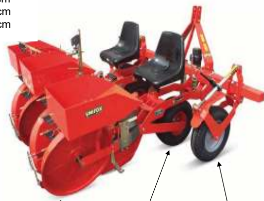
Individual row unit Drive Floating transplant row unit Adjustable support wheel
