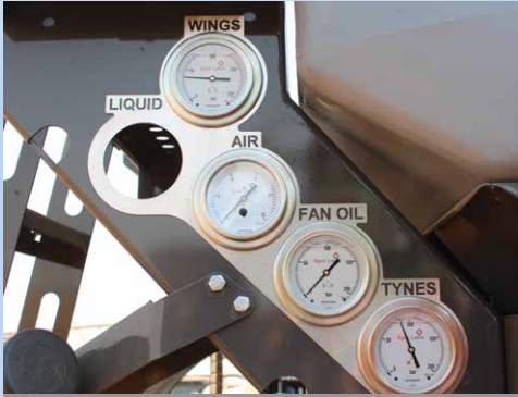
Gauges mounted in central location to be visible from the cab.
