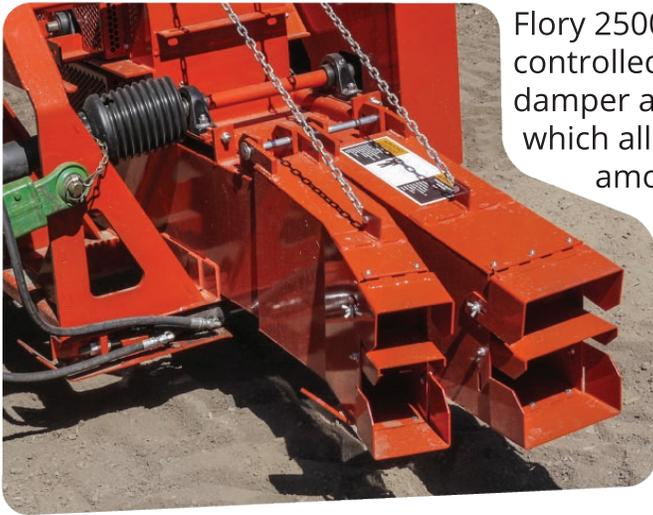
Flory 2500 Blower is controlled with a damper and cylinder which allows a variable amount of air without affecting the R.P.M. of the tractor's engine.
