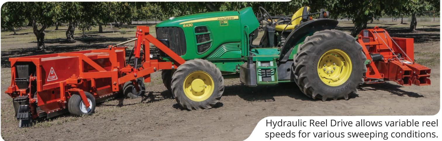
Hydraulic Reel Drive allows variable reel speeds for various sweeping conditions.
