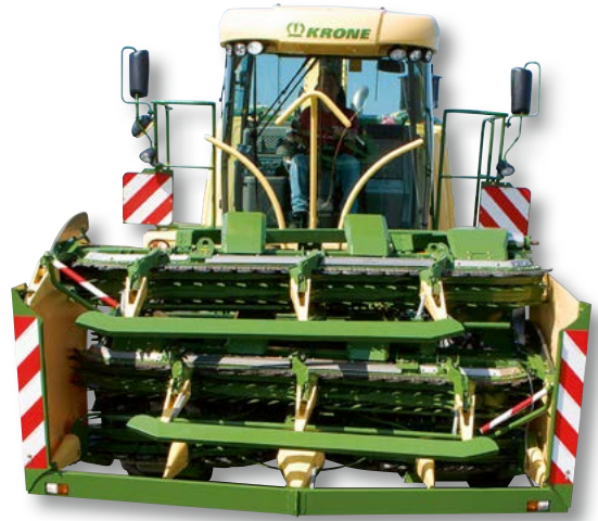
Compact transport position: The triple-fold EasyCollect header
