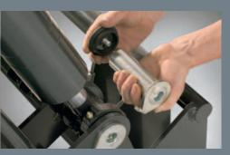
**STRONG AND SMART IN EVERY DETAIL.** All pins are galvanised and are equipped with Quicke's unique pin lock. The tool carrier has extra strong pins where stresses are particularly great. A hinged locking plate with a compact rubber ring prevents axial play, keeps the lubrication grease in place and fixes the pin on both sides.
