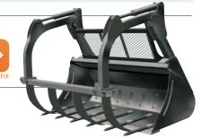
if the loader is without parallel linkage or for tractors without a cab. Maxi Grapple is used particularly in the US and Canada for handling round bales (large 2 m opening), loose hay, brash and branches, loose silage, manure and for bucket work generally. Teeth, protective mesh and the grapple arm are easy to remove when you need to use just the bucket.
