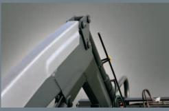
**COMPACT IMPLEMENT INDICATOR.** The position indicator is compact so that it doesn't stick up and cause damage or become damaged itself. It is easy to fit and can be adjusted in three positions for various implements, ensuring exact precision of the implement's angle with the ground.
