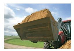
Naturally it has been our aim to design and produce a bucket that does not allow spillage. What is the point of having a large volume bucket if you cannot fill it properly, or if material spills out of it? Therefore our buckets have sides that are laser-cut. The result is a bucket design where the rear edge and the front edge in particular are especially high. It is now possible to fill the bucket completely. You have complete control of the material, and the bucket does not spill any material.
