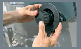
LOCK & GO ENHANCES YOUR SAFETY. Try to find a more convenient connect and disconnect system than Lock & Go. This innovation will save you time without having to compromise on safety. There are no loose parts and no tools are required. You simply connect and disconnect the loader with the minimum possible effort.
