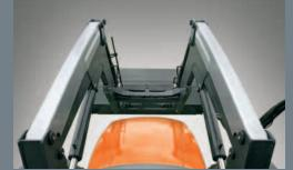
**SIGHT-OPTIMISING DESIGN.** No pipes or hoses that restrict your view. No dirt or rubbish that can accumulate, even if you fit extra equipment to your loader. These are the obvious advantages with Q Vision, where all pipes and hoses are protected in the loader arm.
