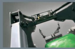
**BENEFIT FIRST AND FOREMOST.** As always at Quicke, the cross tube is located far forward on the loader. This offers a number of advantages. For example, more space for the front linkage and a better view of the implement. The loaders can also be fitted further back on the tractors which increases stability and gives better driving
