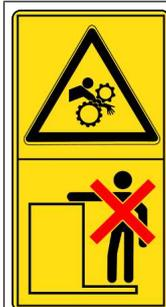
**Danger due to rotating machine parts**
