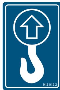
The lifting points on the machine are marked with this label, [see Page 179](#).
