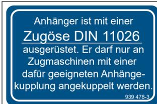
The trailer is equipped with a drawbar eye to DIN 11026. It may only be coupled to tractors with a suitable tow coupling.
