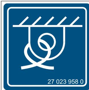
There are lashing points on the machine that are identified with this label, [see Page 180](#).
