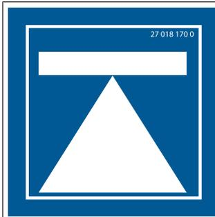
There are jacking points on the machine that are identified with this label, [see Page 235](#).
