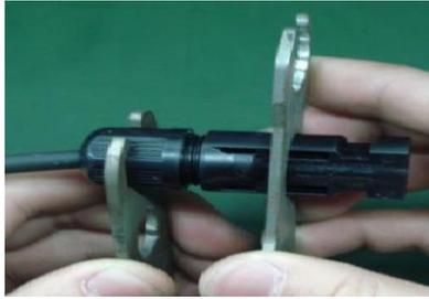
The reference Nut cap locking force is 2.0~2.5Nm.
