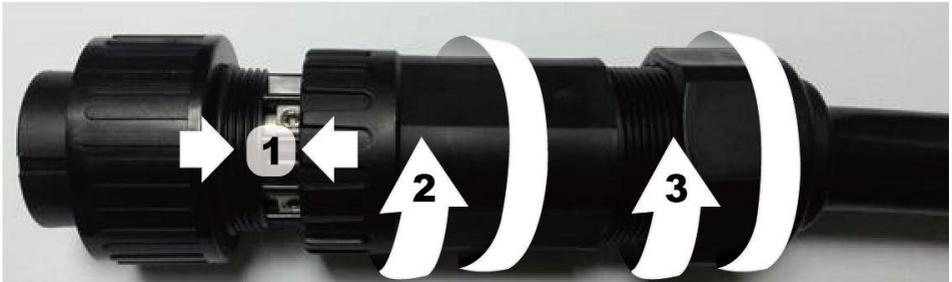
Step 7: Plug the Generator connection socket into GENERATOR terminal of the inverter.
