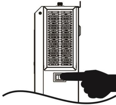
Once the unit has been properly installed and the batteries are connected well, simply press On/Off switch (located on the button of the case) to turn on the unit.
