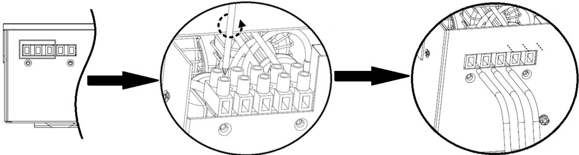
**WARNING:** Be sure that AC power source is disconnected before attempting to hardwire it to the unit.
