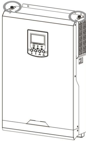
**Step 2:** Then, dustproof case can be removed and take out air filter foam as shown in below chart.
