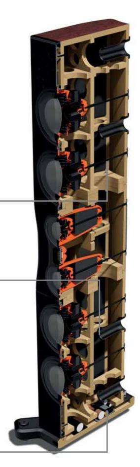
**CURVED AND BRACED CABINET CONSTRUCTION:** Curved surfaces are inherently stronger than flat surfaces, and since the internal sides are non-regular, standing wave formation is suppressed. New internal bracing structures have been developed to ensure the ultimate in structural integrity, and bitumastic damping material applied to all internal cabinet walls to ensure that all cabinet vibration is absorbed. Result: a supremely rigid, acoustically inert enclosure for natural, true-to-life fidelity.
