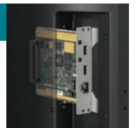
An optional board can slide into the slot on the back of the monitor.
