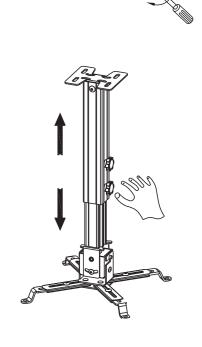
Loosen the locking screw on the Swivel unit holder to adjust projection angle of Projector. Tighten the screw after adjustment.
